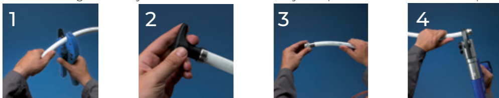
1 Cut the tube. 2 Calibration-beveled tube. 3 Assembling accessory. 4 Press.
